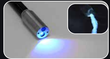
Oil contamination in water showing up white using UVIN
