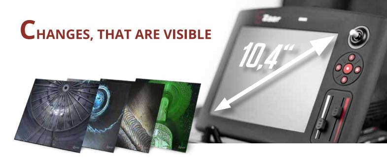
Measuring 10.4", the VUSCREEN is the largest touchscreen on the market of inspection systems. Its PPE compatibility, the shock resistant housing, the intuitive joystick control and numerous image editing options are now joined by an enlarged color space, increased luminance of 850 cd/ $m^2$  and a higher resolution of 1,440 x 1,080 px. Benefit from even brighter and clearer inspection images in particularly natural color representation.
