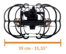
A drone with a small diameter is more maneuverable and better suited for flights in confined spaces. With a diameter of less than 40 cm, the Stereo2 is able to pass through most manholes.
